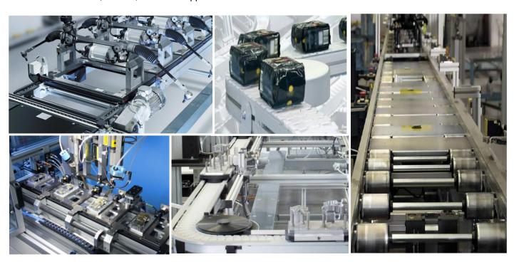
Rexroth have two conveyor product systems, the TS Range of conveyors for pay loads ranging up to 300kg and the VarioFlow flexible chain link conveyor .
