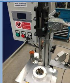
Turbo compressor wheel Induction heater, heating of the bore for shaft pressing.
