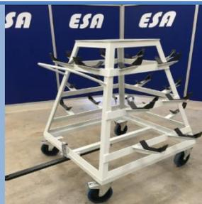
New line side bespoke crank shaft trolleys for a large engine manufacturer client.
