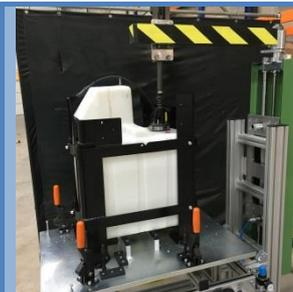
Fuel Tank Assembly station for road sweeper engines.
